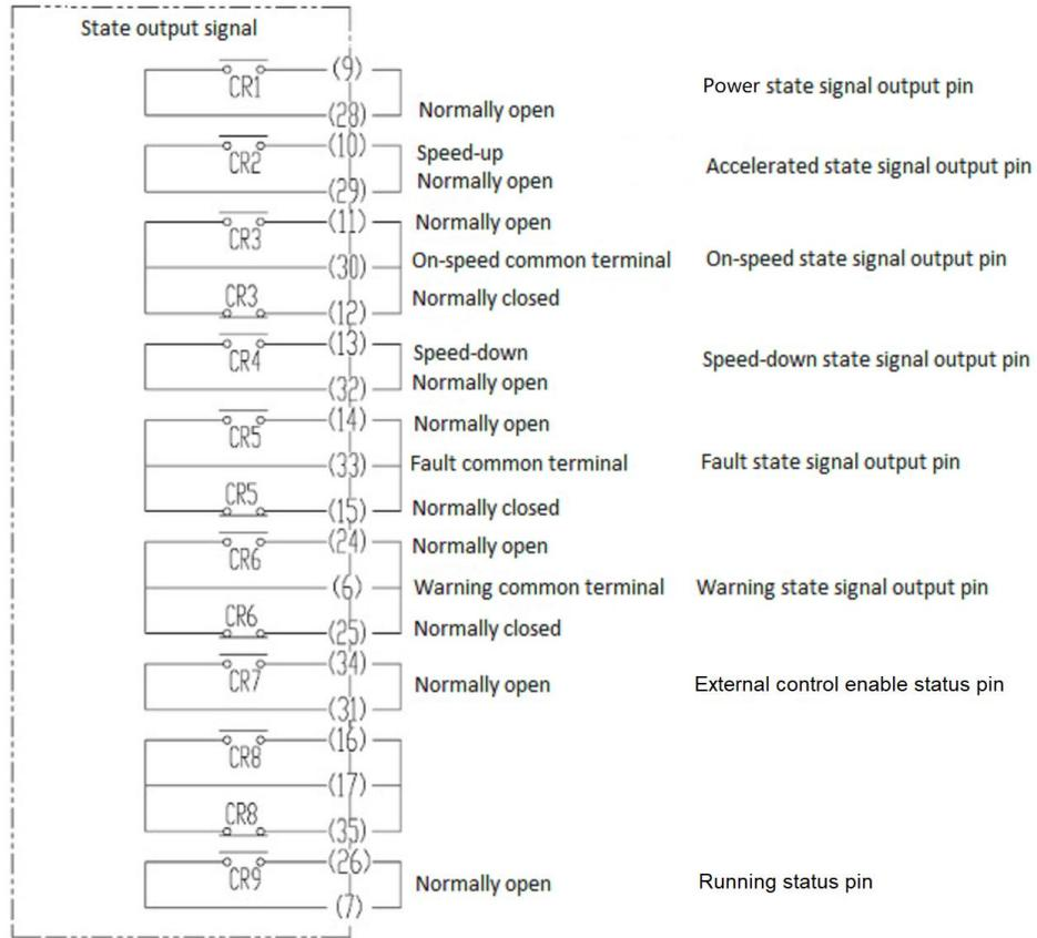
Figure 7.5 Status output signal pins
