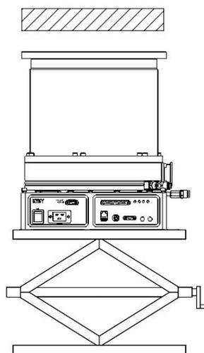
Figure 6.2 Diagram of turbomolecular pump up and down during vertical installation
