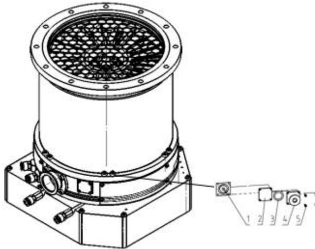
Figure 6.12 Protective gases connections
