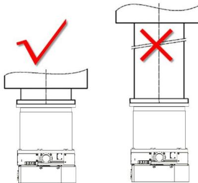
Figure 6.5 Connection diagrams of integrated magnetically-levitated turbomolecular pump and
