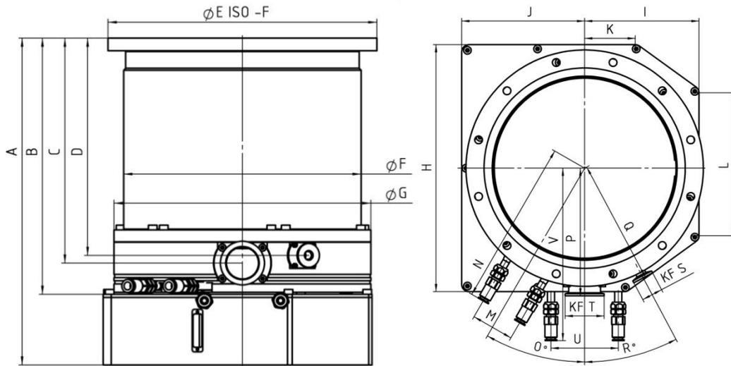
Figure 4.1 Dimensions for CXF-200/1401, CXF-200/1402, CXF-250/2301, CXF-250/2302, CXF-320/3001 and CXF-320/3002
