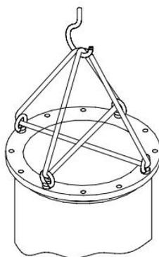
Figure 5.1 Schematic diagram of turbomolecular pump transported by ring screw
