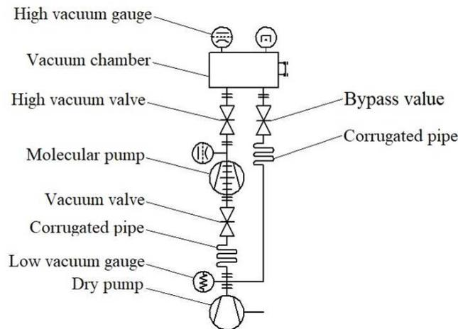
Figure 1.1 Turbomolecular pump applications (vacuum system principle diagram)
