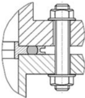
Prior to the flange installation, prepare installation tool, center support, rubber ring, hexagonal bolt and nut, etc. Check the flange sealing surface to ensure that there is no damage;
