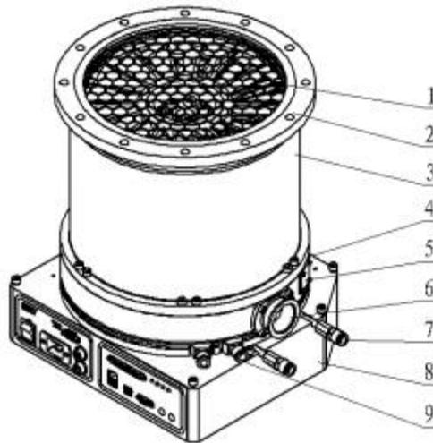
Figure 3.1 Main functional interfaces of turbomolecular pump
