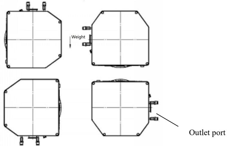
Figure 6.4 Diagram of installation angle of outlet port of integrated magnetically-levitated turbomolecular pump
